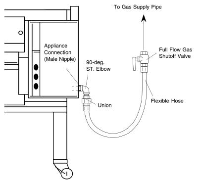
Figure 2-13. Flexible Hose Installation
